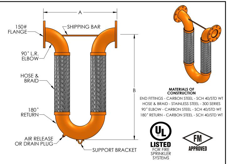
NOTE: METRALOOPS 2" AND LARGER INSTALLED IN ANY ORIENTATION OTHER THAN HANGING DOWN <u>MUST</u> HAVE THE 180° RETURN SUPPORTED. (SEE INSTALLATION INSTRUCTIONS.)
